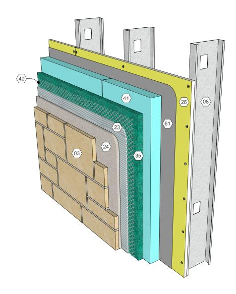
Adhered stone veneer over steel studs backup, rigid insulation, drainage material Wall 03.080.0211 Rev. 11/23/15
