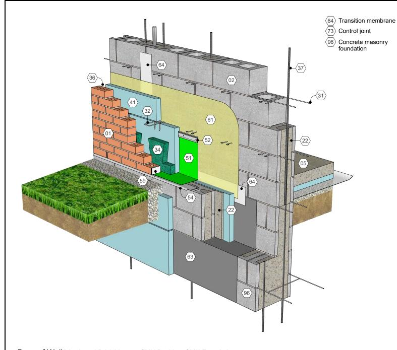
Base of Wall | Anchored Brick Veneer, CMU Backing, CMU Foundation
