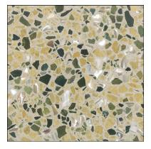
The evolution of terrazzo from a cementitious system to epoxy brings a new concern: controlling moisture. While the cement system developed centuries ago allowed moisture to naturally migrate from the ground or concrete slab and then escape, epoxy-based terrazzo systems do not breathe. That means that if the concrete slab or space below is not controlled, and moisture rises up, epoxy terrazzo will usually fail.
