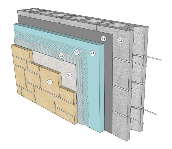
WALL SYSTEM Adhered stone veneer over CMU backup, cont. insulation Detail 03.070.0201 Rev. 10/20/15
