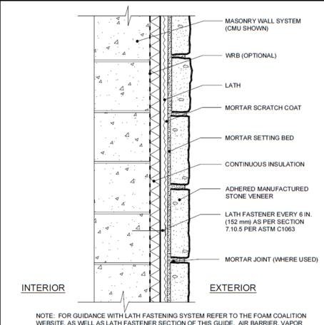
NOTE: FOR GUIDANCE WITH LATH FASTENING SYSTEM REFER TO THE FOAM COALITION WEBSITE, AS WELL AS LATH FASTENER SECTION OF THIS GUIDE. AIR BARRIER, VAPOR BARRIER, WATER-RESISTIVE BARRIER, WATERPROOFING MEMBRANE, FLASHING, LATH ATTACHMENT, Z-CHANNEL, AND INSULATION TYPE AND LOCATIONS TO BE DETERMINED BY DESIGN PROFESSIONAL
