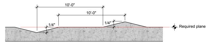
Concrete floor flatness for tile < 15 in. on one side 1/18" in 10 ft., max.
