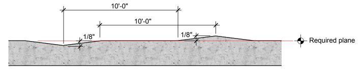
Concrete floor flatness for tile ≥ 15 in. on one side 1/14" in 10 ft., max.
