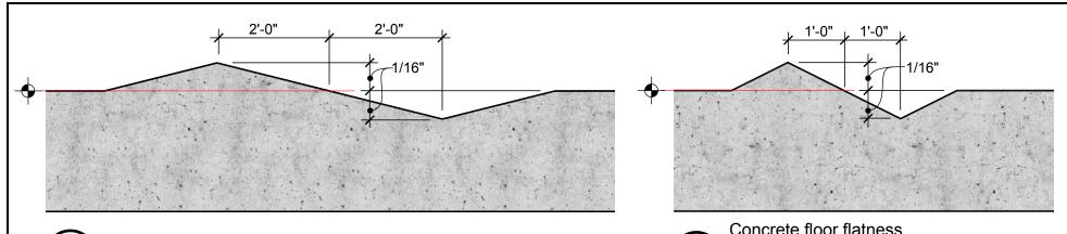
Concrete floor flatness for tile ≥ 15 in. on one side 1/16" in 2 ft., max.
