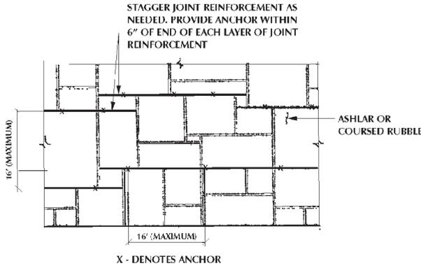
**Figure 6 - Joint Reinforcement (Seismic Design Categories D, E, and F)**
