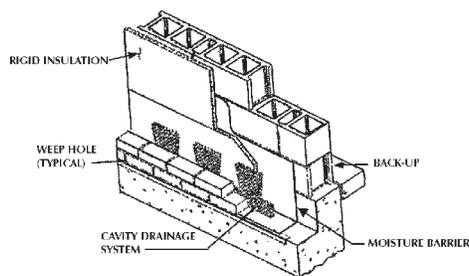
Figure 2 - Cavity Drainage System
