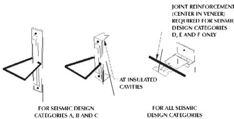
**Figure 5 - Stone Veneer Ties and Anchors**
