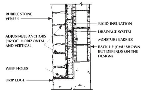
**Figure 9 - Insulated Section**
