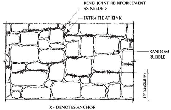
**Figure 7 - Joint Reinforcement (Seismic Design Categories D, E, and F)**
