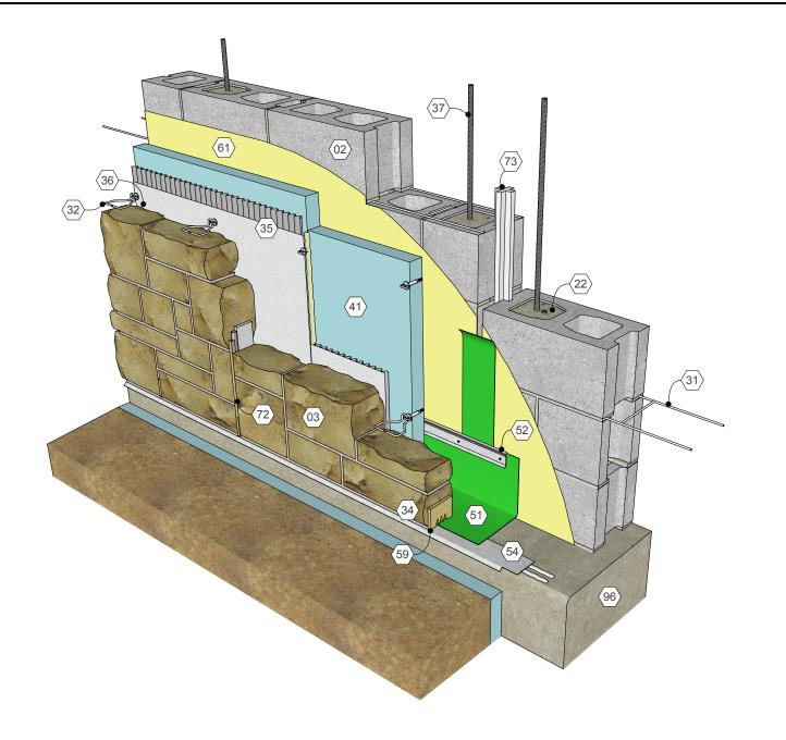
BASE OF WALL Flexible flashing, drip edge, termination bar, drainage mat Detail 03.030.0101 7/28/16
